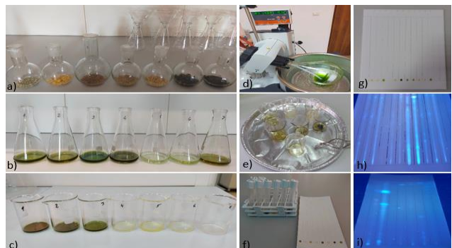
Figure 5. Working technique (a-degreasing of samples; b, c-cold extraction; d, e-dry evaporation in rotavapor; f, g-plate staining; h, i-mycotoxins identified)
