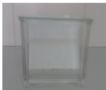
Figure 2. Chromatographic plate in the developing solvent
