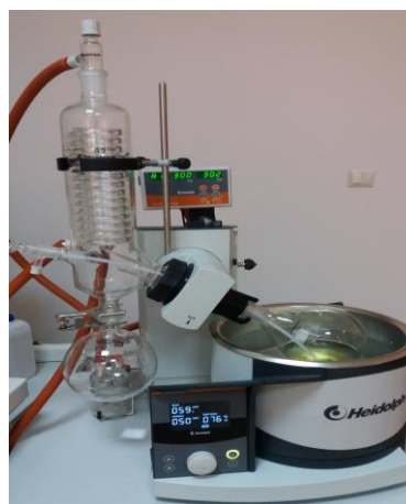
Figure 1. Dry evaporation at the rotary evaporator
